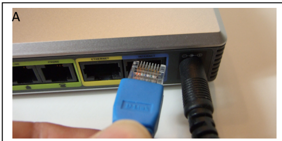
A Connect the Ethernet cable with router or modem, and the supplied power adaptor.
