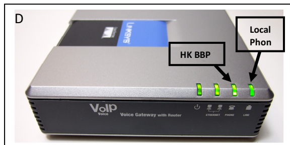
D The first 2 indicator lights should be on and blink. When the 3 rd & 4 th indicator lights turn on, means the HK BBP or Local phone are ready to use.
